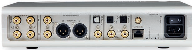
ABOVE: Four S/PDIF and two RCA analogue inputs should be adequate for most requirements. Power amp connection can be balanced (XLR) or single-ended (RCA)
